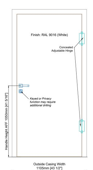
145mm [5 11/16"] Outside Casing Height AFF 2177mm [85 11/16"] Finished Opening Height AFF 2094mm [82 7/16"] Finished Door Height 2097mm [82 9/16"] RO 2146mm [84 1/2"] +/- 20mm [13/16"] 7mm [1/4" 40mm [1 9/16"]
