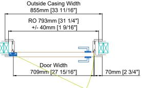
\*120mm [4 3/4"] \*Jamb thickness up to 145mm [5 11/16"] Outside Casing Height AFF 2177mm [85 11/16"] Finished Opening Height AFF 2094mm [82 7/16"] Finished Door Height 2097mm [82 9/16"] RO 2146mm [84 1/2"] +/- 20mm [13/16"] 7mm [1/4"] 40mm [1 9/16"]
