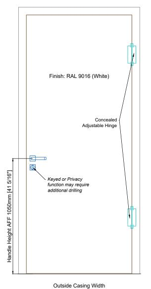
\*Jamb thickness up to 145mm [5 11/16"] Outside Casing Height AFF 2427mm [95 9/16"] Finished Opening Height AFF 2344mm [92 5/16"] Finished Door Height 2347mm [92 3/8"] RO 2396mm [94 5/16"] +/- 20mm [13/16"] 7mm [1/4" 40mm [1 9/16"]
