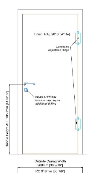
Outside Casing Height AFF 2177mm [85 11/16"] Finished Opening Height AFF 2094mm [82 7/16"] Finished Door Height 2097mm [82 9/16"] RO 2146mm [84 1/2"] +/- 20mm [13/16"] 7mm [1/4"] 40mm [1 9/16"] T R A D E M A R K C O L L E C T I O N
